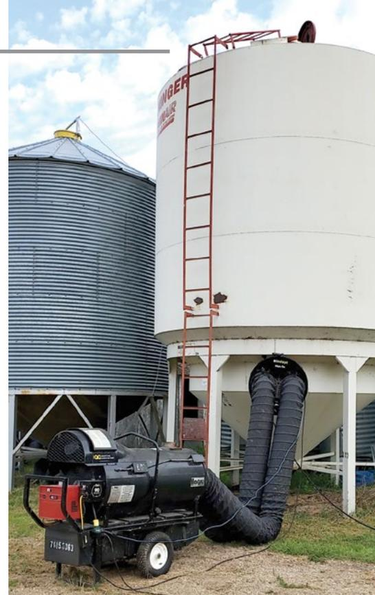
Above: Shawn Senko uses his 400,000-btu diesel supplemental heater to boost the drying capacity of his aeration fans. The lower up-front cost and ability to move it from bin to bin make these supplemental heaters an attractive drying option.
